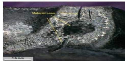
Fig. 5 Hollowing out of a polyacetal hinge due to acidcatalyzed Hydrolysis. [2]
