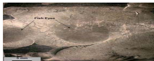
Fig. 6 Hydrogen damage of induction-hardened steel piston rod displaying fisheyes. [2]
